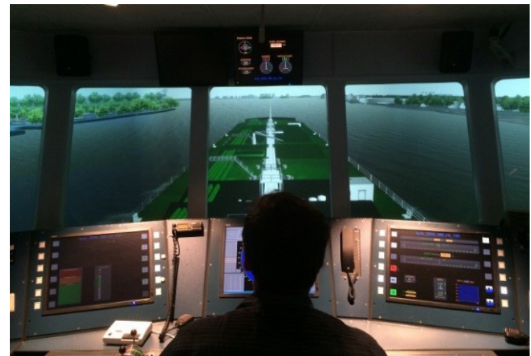
Scale models of different hull forms (L) and ship manoeuvring simulator with mud inputs (R)
