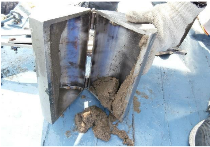
Bed sampling with a 'Van Veen' grab (L) and lab analysis for grain size distribution (R)
