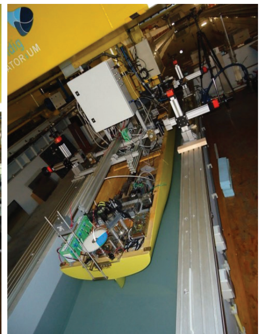
Towing tank with a scale model to be towed by the overhead gantry.
