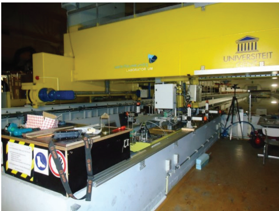
Towing tank with a scale model to be towed by the overhead gantry.
